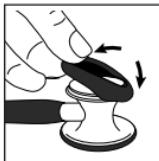
Attach the sleeve by placing one side on the edge and stretching it over the chestpiece.
