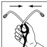
To increase the spring tension, squeeze the eartubes together.
