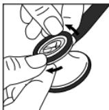
To install diaphragm, remove the nonchill sleeve. Insert the edge of the diaphragm into the groove and roll the rim around the chestpiece.
