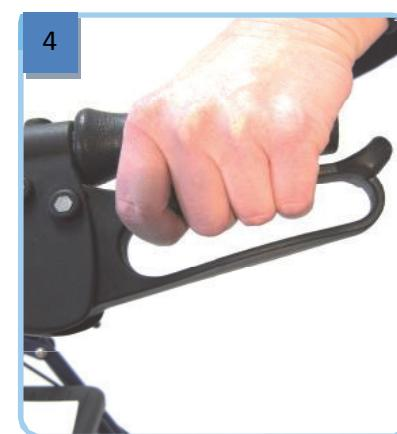
For breaking the walking device pull both brakes upwards to the handgrip (see picture 4). Always brake slowly and steady.
